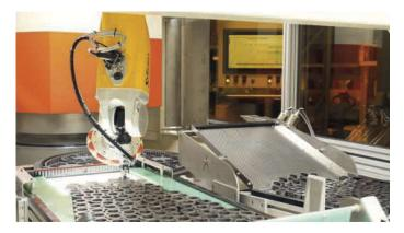
unoriented workpieces into a correct orientation in the carriers mounted in the machine. There is a magnetic head attached for fast unloading, but piece-by-piece unloading would also be possible when required. For example, measuring parts externally before unloading the batch.
